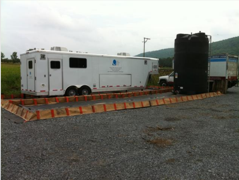
Figure 2B shows the mobile laboratory on its environmental protection apron at the field site. The large black poly tank contains waste fluids
